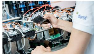
Simple Exchange of Printheads When necessary, the Alpha Printheads can be exchanged by the operator within a minimum amount of time, thus minimizing down-time.
