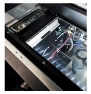
**Ouick Purging Cycle** The Purging Station will affect a complete and automated cleaning of the nozzles within 160 seconds. This new purging concept also allows for individual color rows to be cleaned.
