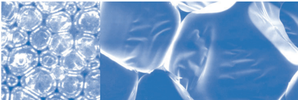
■ A stability principle derived from nature: the networked honeycomb structure of the KAPA® polyurethane hard foam core seen under a microscope.
