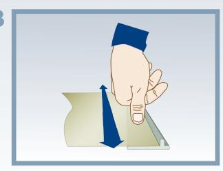
Remove the remaining part of the protective liner and press the image firmly onto the panelstrip.
