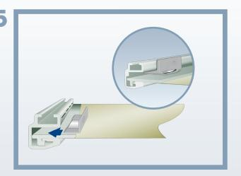
Turn the image around and push the clips into the places marked with a black line at the top profile.
