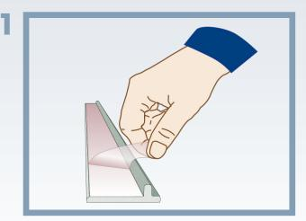
Remove a small part of the protective liner on the tape.
