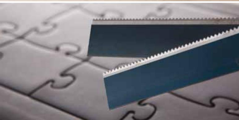
KAPA® boards can be processed and transformed into a wide variety of shapes and original objects on all standard die cutting presses.
